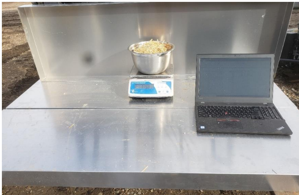
Figure 6. Weighing crop residue material for size distribution analysis.
