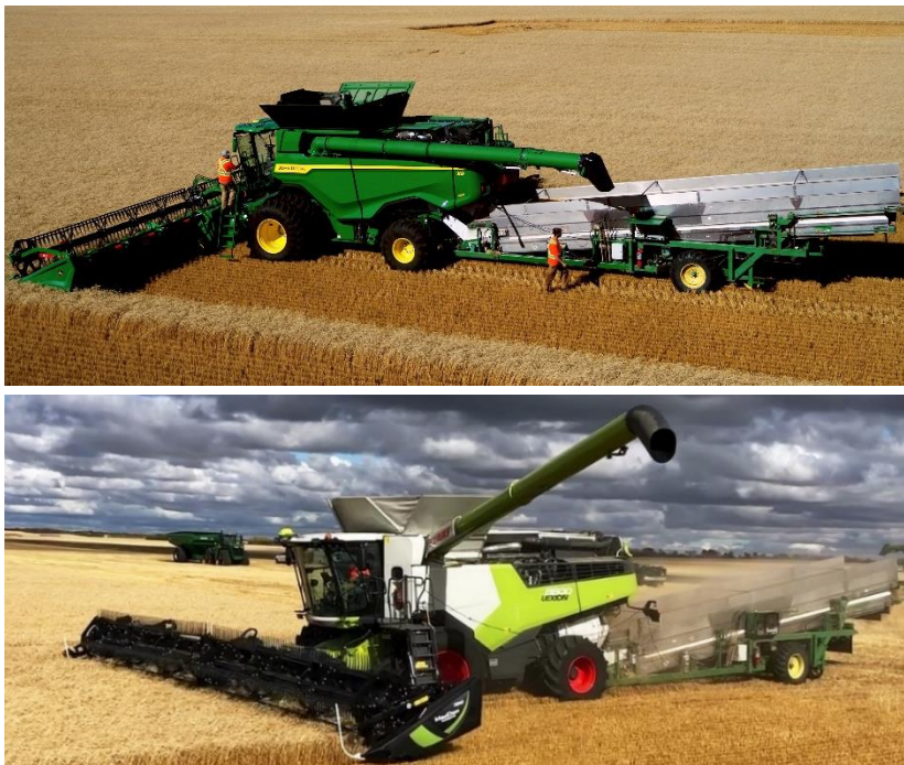
Figure 1. John Deere X9 (top) and CLAAS Lexion 8800 (bottom) towing collector during loss curve testing.
